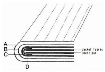
How to check the hardness of the collar (after washed and dried)
