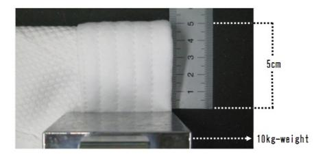
The height (width) of collar folded into two must be within 4cm.
