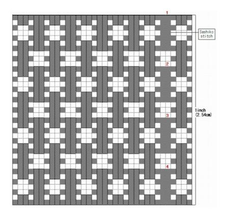
**Note:** If fabric has not enough Sashiko yarns, it becomes softer and easy to be stretched causing difficulty for applying technics (Waza). On the other hand, if fabric has excess of Sashiko yarns, it becomes harder causing difficulty of handgrip.
